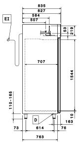
ED Remote electrical connection RO Refrigerant Outlet
